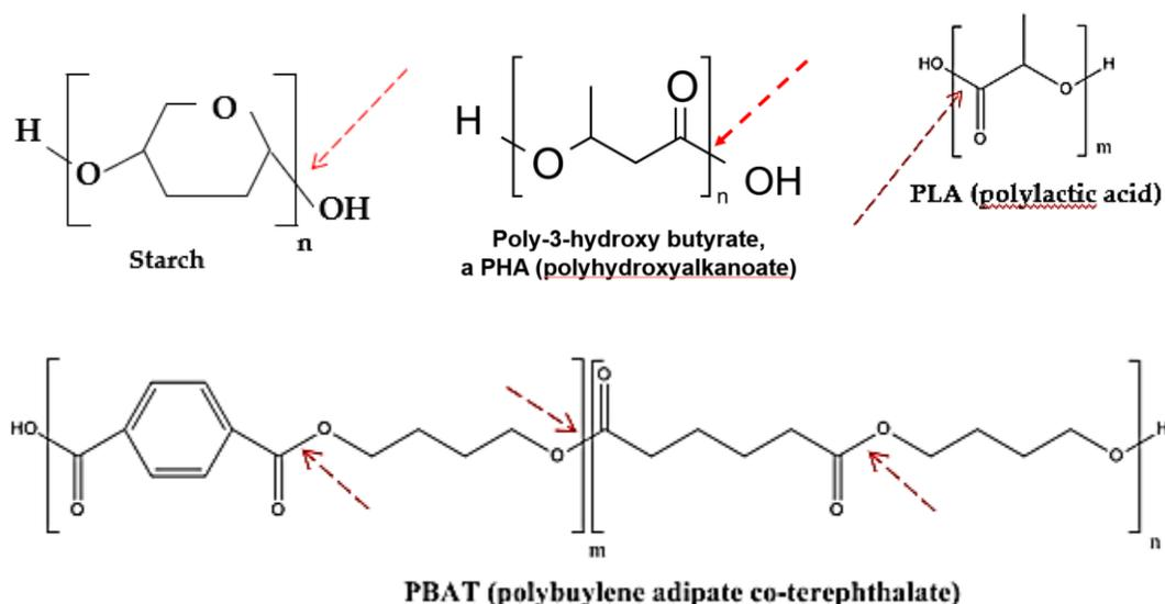
Figure 2. Molecular structure of commonly used polymeric components for biodegradable mulch films. Red arrows indicate hydrolyzable chemical bonds that undergo breakdown during microbial attack.
