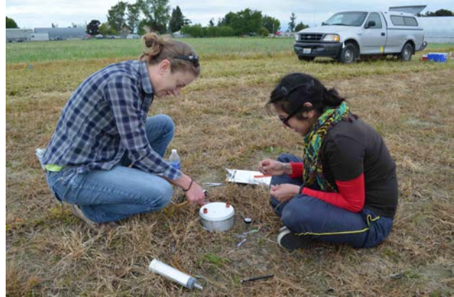
Figure 1: Soil respiration measurements with a closed chamber inserted into the soil.
