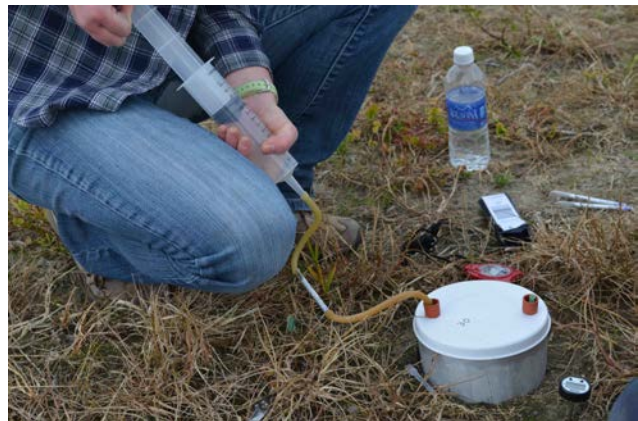
Figure 2: CO 2 is pulled through a measurement tube with a syringe.
