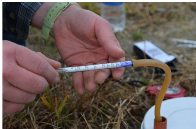
Figure 3: Coloration indicates the CO 2 concentration in the soil air.
