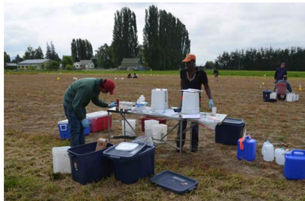
Figure 5: Soil pH, electrical conductivity, and nitrate measurements in the field.
