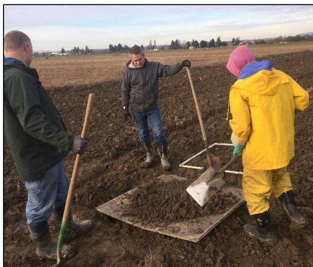
Figure 2. Collection of a soil sample from an area of 3 ft by 3 ft (9 ft 2 ) and depth of 6 in. using a shovel and placed on a piece of plywood ( \geq 4 \text{ ft} \times 4 \text{ ft} ).
