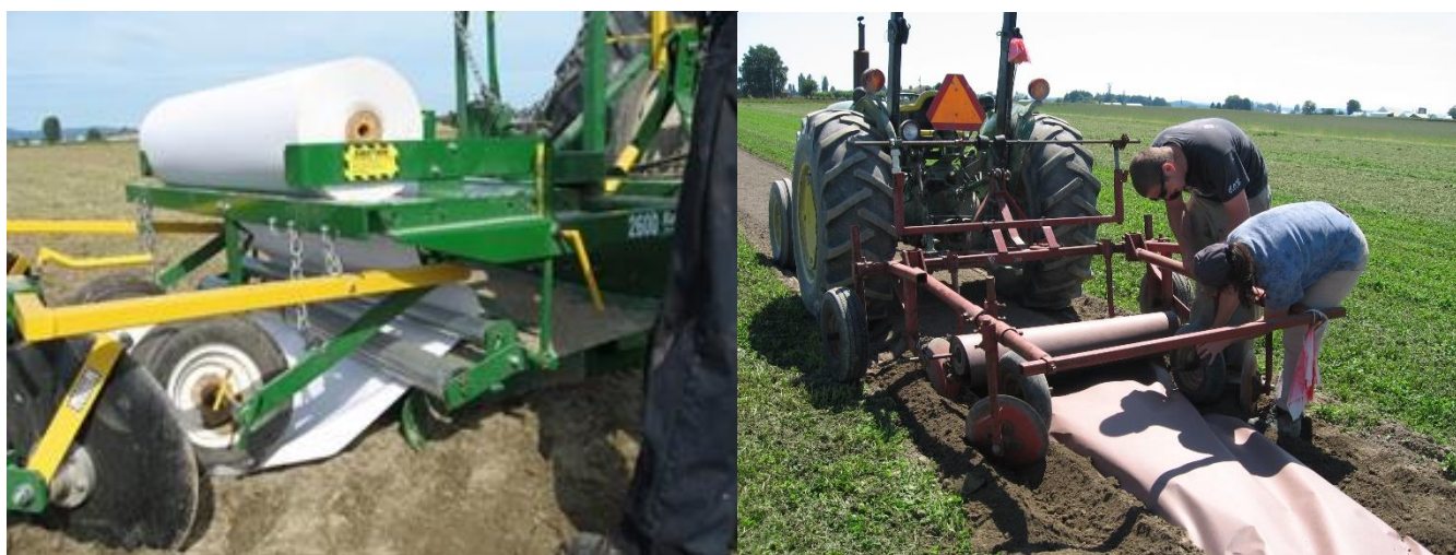
Figure 2. Biodegradable paper mulch on a raised-bed mulch layer, showing placement under the roller bars (left), and on a flat-bed mulch layer (right). (Photos: C. Miles.)
