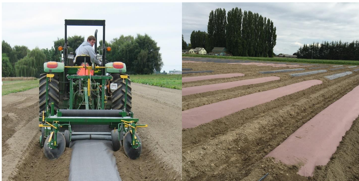
Figure 1. Laying plastic BDM with a raised bed shaper (left); paper BDM laid by machine (right). (Photos: C. Miles.)
