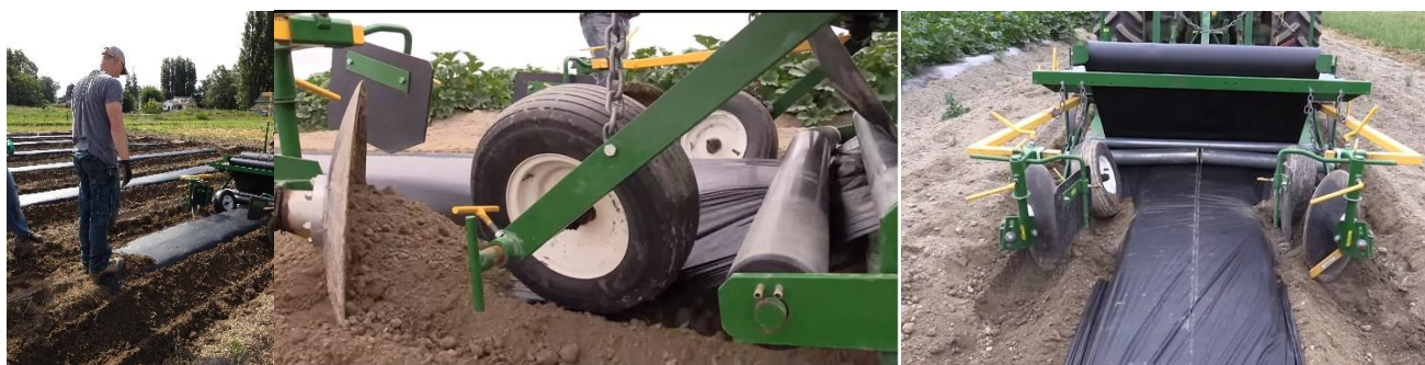
Figure 3. Step on the mulch before the tractor starts moving forward to hold the mulch in place (left). Mulch layer roller bars should move freely and wheels should barely touch the mulch (middle). The mulch should be laid loose on the bed to avoid ripping (right), and when the mulch is moistened and then has dried, it will become tight across the bed. (Photos: S. Ghimire.)
