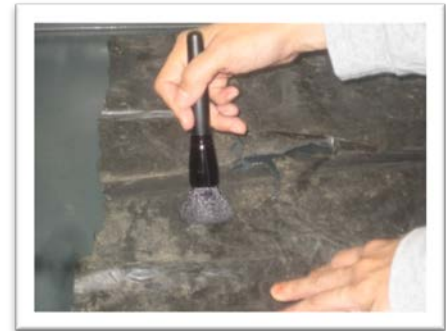
Before being subjected to the tensile strength assessment, the biodegradable plastic mulch samples retrieved from the field test site are cleaned through careful brushing with a soft bristle brush.
