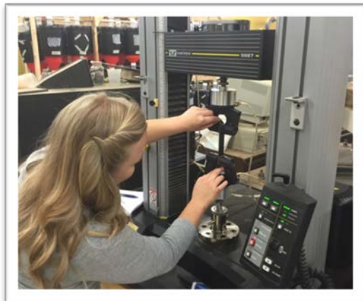
A research assistant affixes the biodegradable mulch sample to the clasps of the tensile strength analyzer. The tests are governed by standardized testing procedures.
